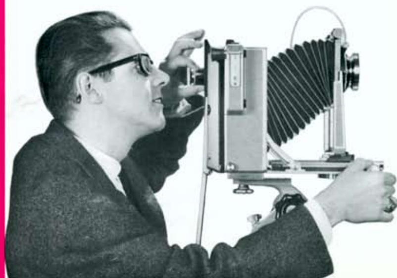
Camera position and lens as above; perspective effect increased by extreme lateral shift of the lens standard to the left. As a result of increased angle of camera back, subject appears considerably extended.
