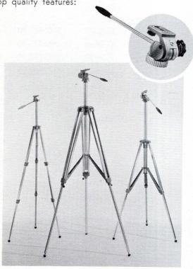
HYDRONALIUM ALLOY. Leg sections are made of sturdy, corrosion-resistant Hydronalium proven in hundreds of thousands of Linhof Precision tripods; each section is ground, polished and anodized to a smooth finish which keeps hands and clothing free from smudges, Hydronalium alloy combines lasting sturdiness with surprisingly light weight.
