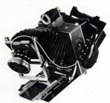
SUPER TECHNIKA 5x7, Model V; new universal swing-and-tilt lens standard with lateral shift; Multifocus rangefinder for all lenses from wide-angle to 500mm telephoto; revolving interchangeable back. Supplied complete with blanklens board, blank distance scale slide, blank rangefinder coupling cam built-in spirit level. Leather grained Sierra Tan finish with chrome trim
